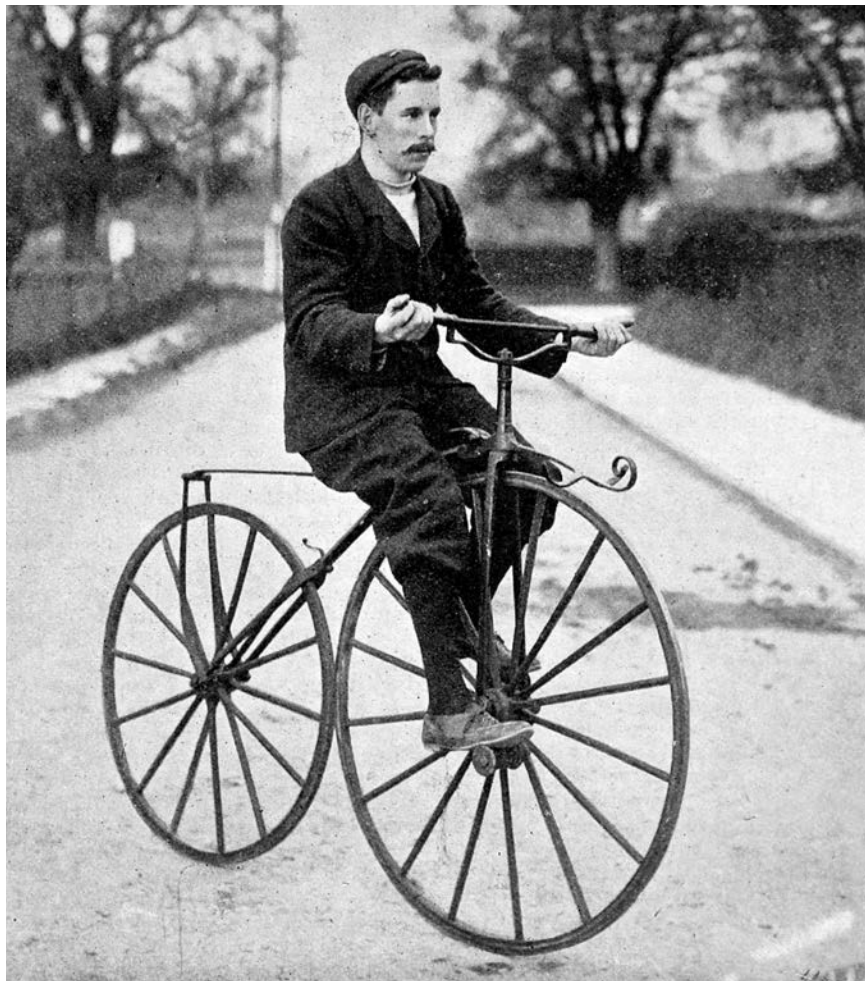
The heavy iron frame and wheels of this bike made the ride so bumpy that it was called the boneshaker .
