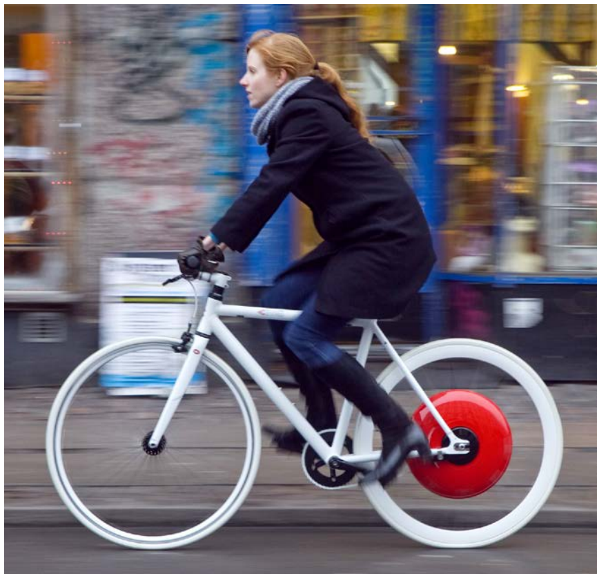
The Copenhagen Wheel can replace the back wheel of most bikes. A motor inside it provides extra power so riders can travel for long distances or up hills.
